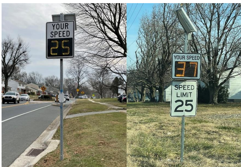
Figure 1: Examples of radar speed signs in Delaware
